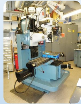
Manual/CNC Mill. We have two. They can make parts like this.
